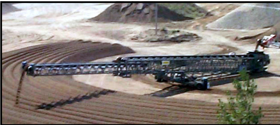
MARCO TELESCOPING RADIAL CONVEYOR
