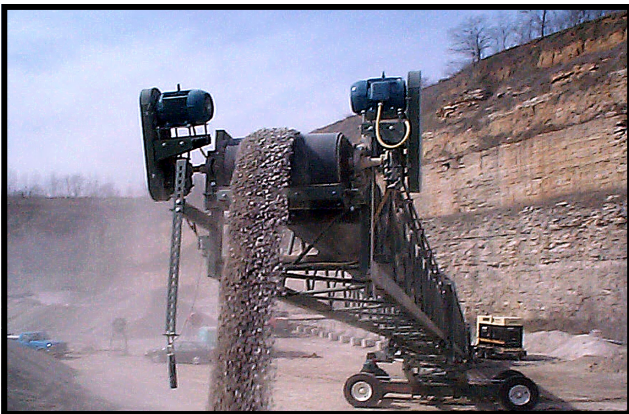
MARCO TELESCOPING RADIAL CONVEYOR
